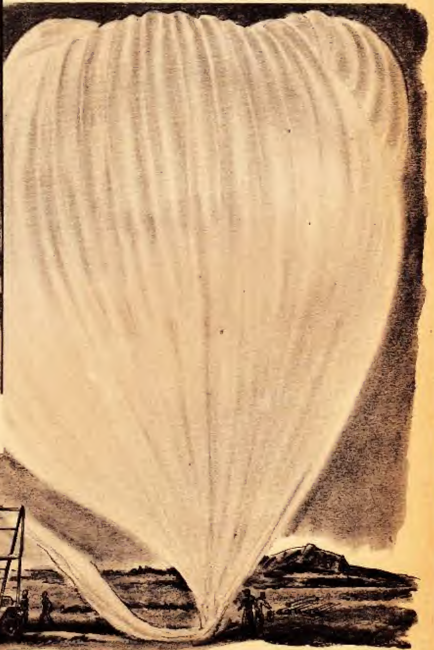
The rocket frame (on a truck) awaits inflation of the plastic balloon.
